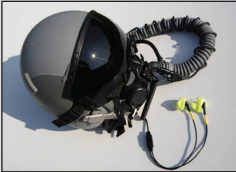
AFRL's newly patented ACCES ® [Attenuating Custom Communications Earpiece System] technology (Air Force image)
